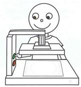
4. 將徽章與膠膜置於機器平台上。設定溫度為100°C。啟動機器,降下熱壓板面。 Leave them on the platform at proper position. Set the temperature at 100°C (about 212°F) Start the machine.
