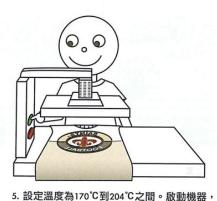
降下熱壓板面。 Set that temperature between 170°C to 204°C (about 338°F to 399°F). Start the hot pressing.
