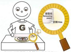
3. 將巨松熱融膠膜完全覆蓋於徽章的背面。 (膠膜的離型紙面需朝上、膠膜面朝下) Fully cover GESONG HSA Film (with the film side down and the releasing paper side up) on the reverse side of the embroidery.
