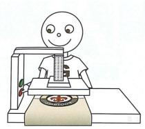
7. 加熱完成,升起熱壓板面。 Heating finished. Stop the machine.
